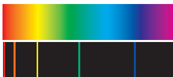
Figure 8.33 A continuous spectrum from a solid and the line spectrum for the gas hydrogen.
