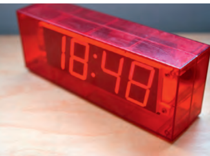
A seven segment LCD – each segment is a separate crystal.
